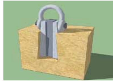
Lewis bolt, the central plug is adjustable
